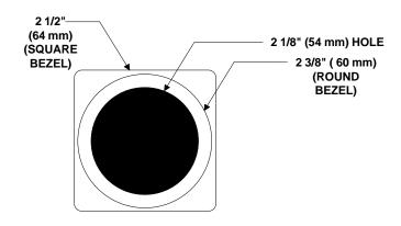
When you determine the location for the unit, drill a 2 1/8" (54 mm) hole in the dash. Slide the unit through the hole from the front of the dash. Align it so that it's straight, then tighten the two screws with a phillipshead screwdriver.
